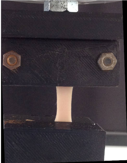
Figure 2: Photo of a rectangular sample demonstrating non-uniform deformation under tension
