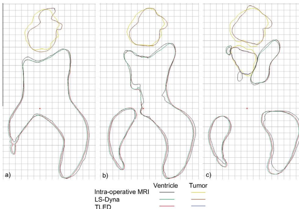
Fig. 3. Brain shift simulation – comparison between the simulation results and the intra-operative MRI. The cutting sections are perpendicular to the superiorly pointing axis, with 0 on the brain's most superior vertex, at distances of (a) -45.5 mm, (b) -50.5 mm and (c) -55.5 mm. Grid lines are 5 mm apart.
